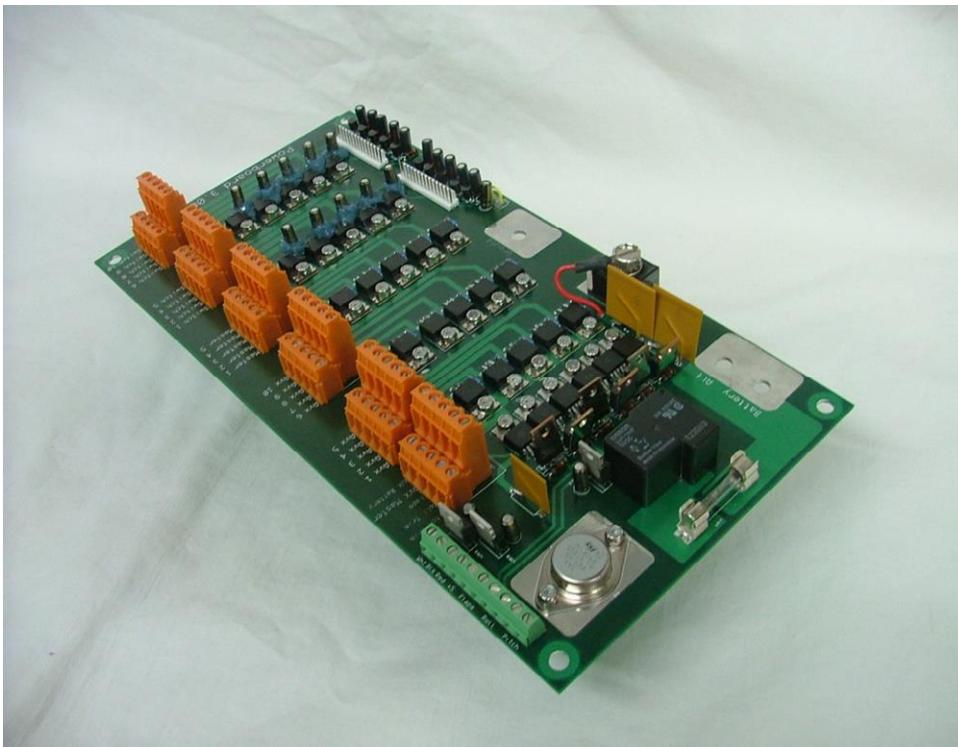
The concept of the Power Board is very simple: provide a place to connect almost everything electrical and connect it safely. The Power Board is extensively fused (circuit protected) with silicon over-current sensors and the main circuit is protected by a 50-amp Slow-Blow fuse. Everything connects to the Power Board except for your starter and high-current loads like HID lights.
